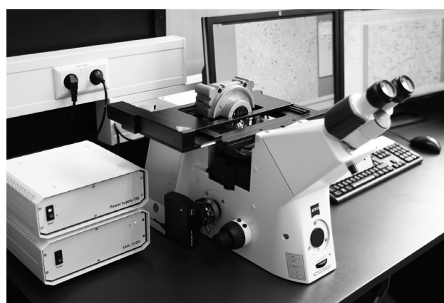
Fig. 1: Microstructural analysis of macrosections of larger nonferrous cast components. The inverse design of the microscope makes it easier and quicker for users to conduct their analysis. Samples do not need to be separated and mounted; those being inspected are positioned directly at focus level, allowing even large and heavy samples to be examined directly.
