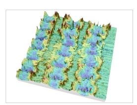
Laser structured surface, 3D view of color coded height map with texture overlay, C Epiplan-Apochromat 50×/0.95
