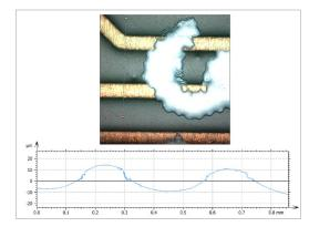
Profile measurement of a circuit board, 3D view with true color overlay, C Epiplan-Apochromat 10×/0.4
