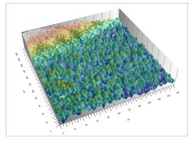
Silver finger on solar cell surface, 3D view of color coded height map with texture overlay, C Epiplan-Apochromat 50×/0.95
