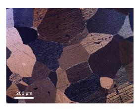
Zinc metal, reflected-light polarization, magnification: 100x
