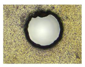
PCB drilled hole inspection, simultaneous reflected and transmitted light
