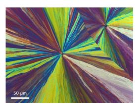
Veranol in crossed polarization with lambda plate, magnification: 200x
