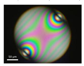
Mylar foil (biaxial-oriented polyethylene terephthalate film), conoscopy, magnification: 400x
