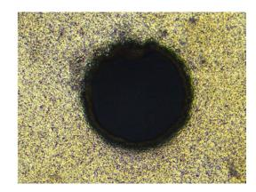
PCB drilled hole inspection, reflected light
