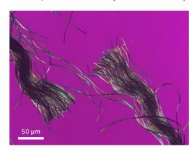
Polyamid, polarization with lambda plate, magnification: 50x
